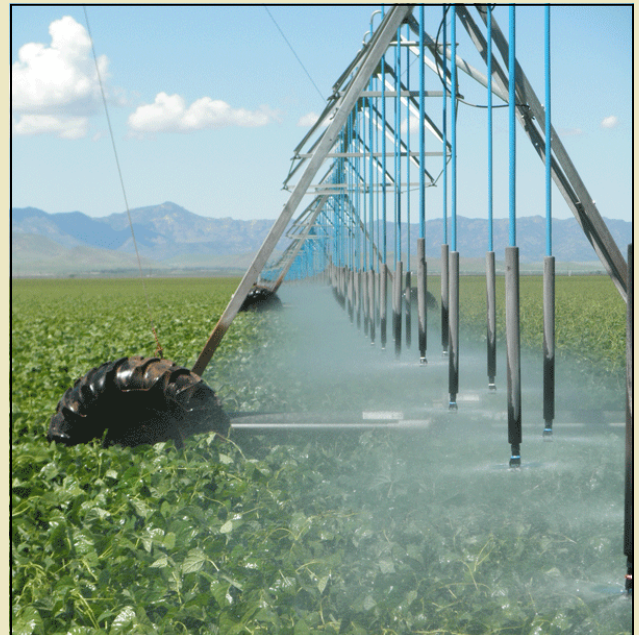
Center pivot irrigation system. Increased evaporation from large-scale irrigation affects local temperatures by increasing relative humidity. Source: NRCS. http://www.az.nrcs.usda.gov/news/releases/Tedd-Haas-Irrigation-Efficiency.html
