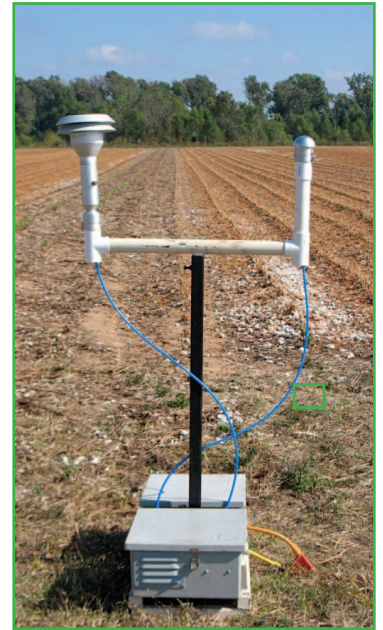
Figure 2. Low-volume PM sampler. The air flow is about 1 cfm.
