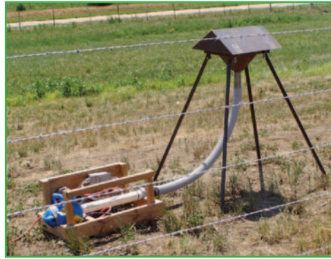
Figure 1. A high-volume particulate matter sampler. Air is pulled through a filter under the rain hood using a vacuum fan at 40 to 60 cubic feet per minute (cfm).
