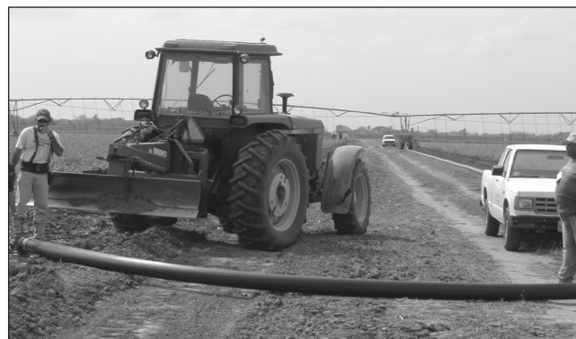
Figure 8. Linear moving system with a flexible hose. Source: Texas A&M University Research and Extension Center at Weslaco.
