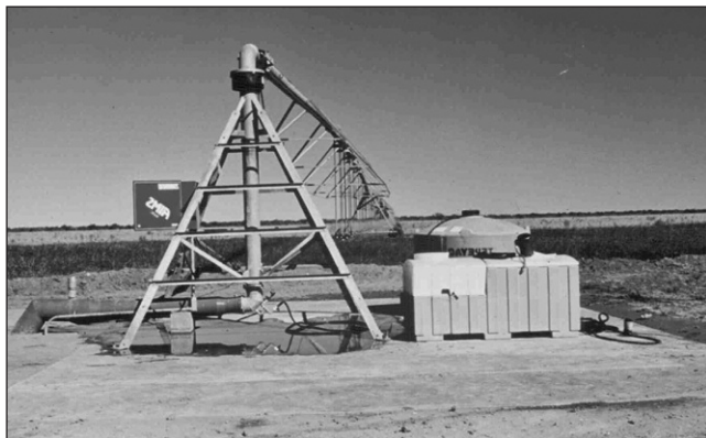
Figure 7. Center pivot sprinkler system.
