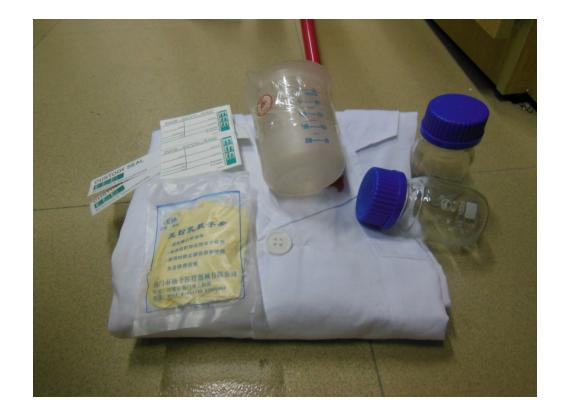
Systematic Random Sampling, based on time intervals, was performed on 3 water sources on campus. Using the dipper, the running water at the locations was collected and placed in glass jars. The jars were labeled after collection and stored:
