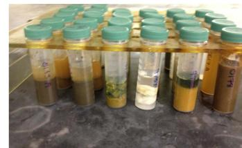
The tests I learned the most about and conducted on my own included measuring and cataloguing the pH of liquids and solids, the conductivity of liquids and solids, and the sulfur content of crude oil. I interned with Ana-Lab for only a short period of time, and these few tests were the least complicated and the easiest to learn quickly.
