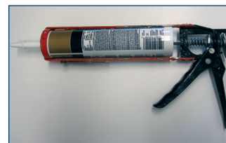
Figure 5. Caulking gun and sealant.
