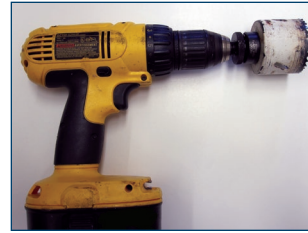
Figure 8. Drill and 2 3/8-inch hole saw.
