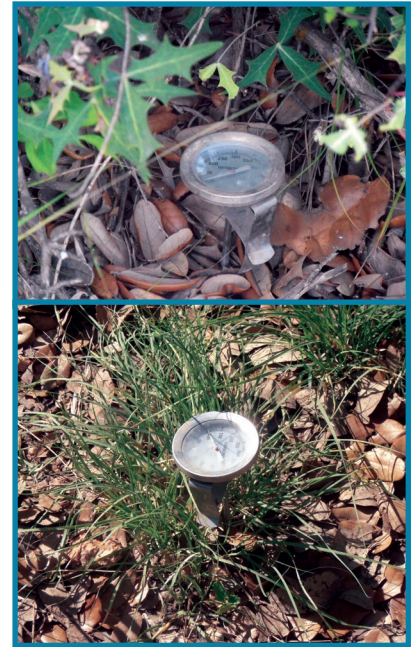
The thermometer on the top is in shade and in litter. The one on the bottom is in full sun and short grass with little litter.
