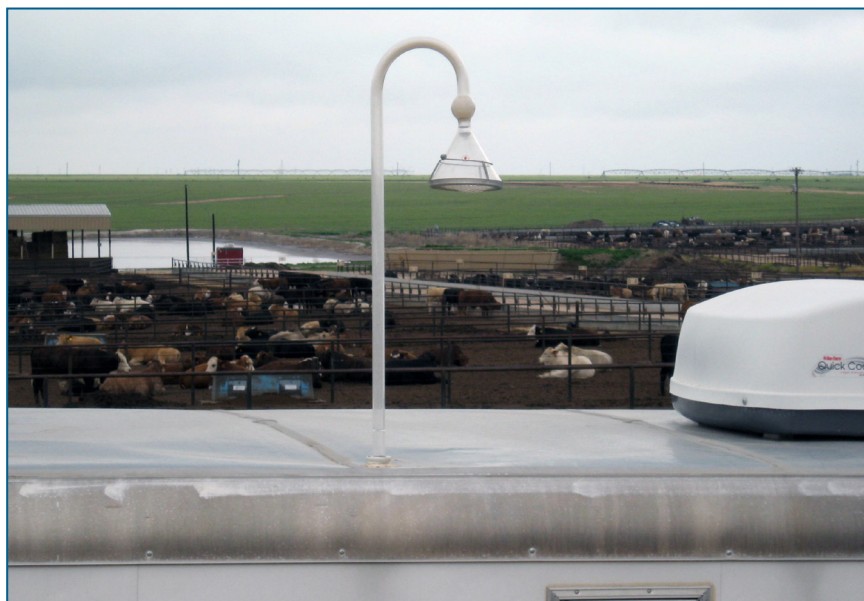
An intake port mounted on the roof of a trailer deployed at a CAFO provides air samples to hydrogen sulfide analyzers inside the trailer. The pen surfaces and runoff holding pond visible in the background are potential sources of hydrogen sulfide. (Photo courtesy of K. Casey)
