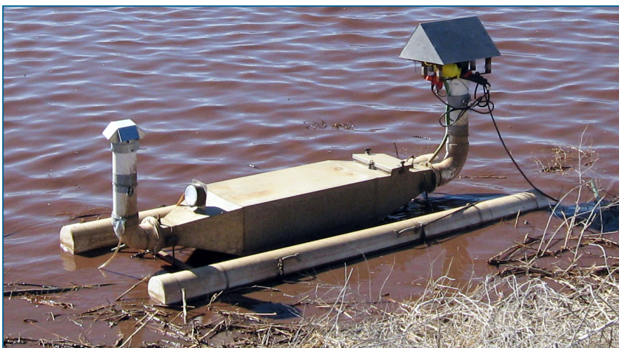
A wind tunnel floating on the surface of a treatment lagoon collects air samples that are sent to a hydrogen sulfide analyzer. (Photo courtesy of K. Casey)
