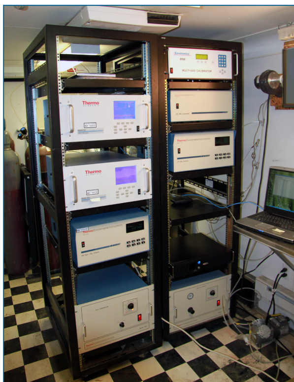
Several gas analyzers operating inside a trailer deployed at a CAFO including two hydrogen sulfide analyzers (Model 450i, left rack, 2 nd from top; Model 45C, left rack, 3 rd from top) by Thermo Scientific (Waltham, MA). (Photo courtesy of K. Casey)
