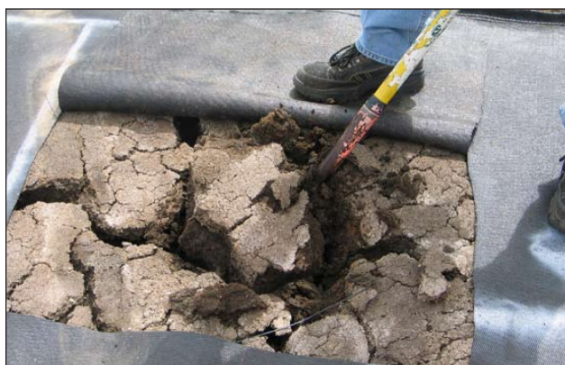
Figure 5: Residual solids in dewatered Geotube®.
