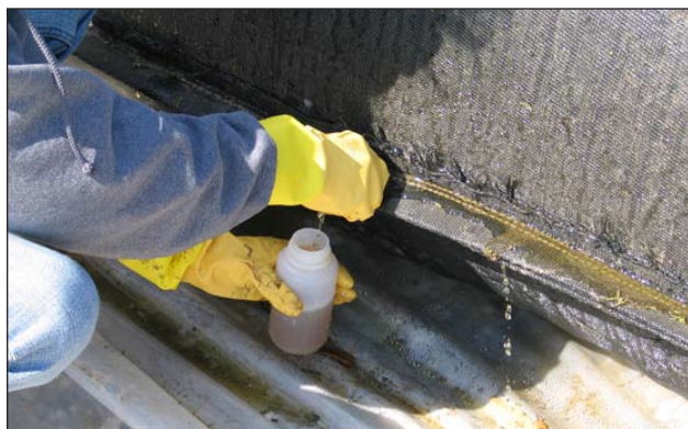
Figure 4: Sample collection from a Geotube®.
