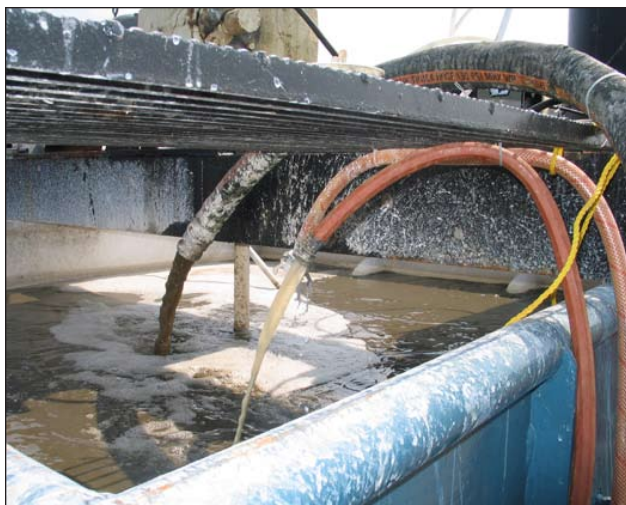
Figure 8: Mixing tank with chemical additions.
