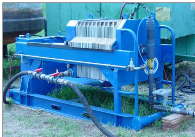
Figure 7: EC unit with iron electrodes built on a filter press frame.
