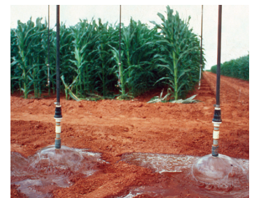
Figure 6. LEPA center pivot with a bubble applicator on corn.
