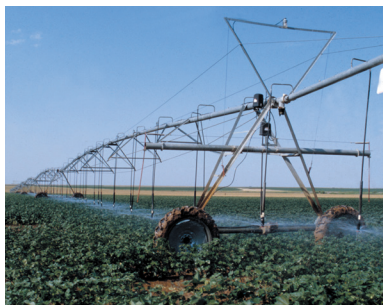
Figure 4. LESA center pivot on cotton.
