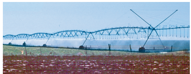
Figure 3. MESA center pivot, half-mile system.
